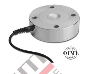
even when side forces are inevitable in normal operations. The typical example for side force resistance is the application in motor truck scales. PSD is constructed of alloy steel and is fully potted with special chemical compounds to IP67 to protect the cell from water and moisture attack.
