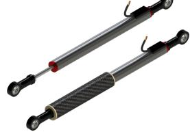
The KP Series of KP13S Standard Light Duty Linear Positon Sensors are designed to withstand the harsh environments within motorsport and automotive testing applications. By using a proven conductive plastic, track technology and multi-fingered contacts, the KP13S offers high performance and reliability under extreme temperature and vibration.
