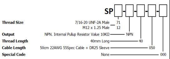
The KA configuration tool is used to specify a standard KA Sensor, other options are available.
