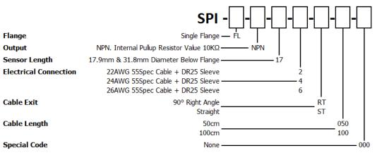
The KA configuration tool is used to specify a standard KA Sensor, other options are available.
