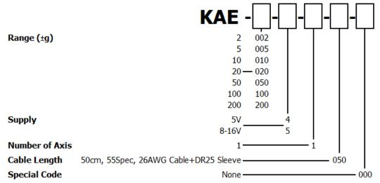
The KA configuration tool is used to specify a standard KA Sensor, other options are available.
