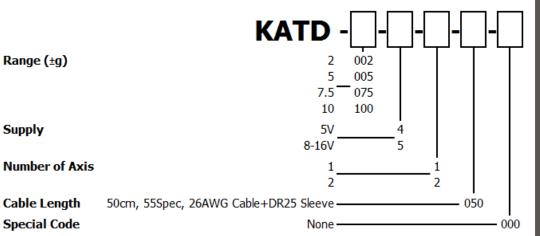
The KA configuration tool is used to specify a standard KA Sensor, other options are available.
