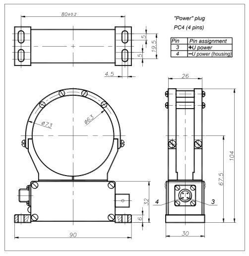
Rotor. Dimensions in mm.
