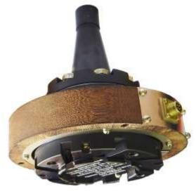
The M44 measures 4 components of force (Fx, Fy, Fz) along the three orthogonal axis (X, Y, Z) and torque (Mz) during the rotating. The M44 can be used for logging of the friction stir weldind (FSW) parameters.
